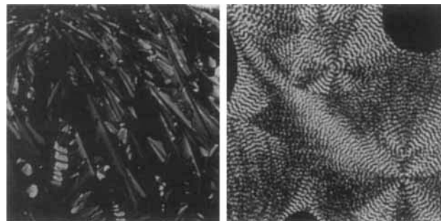
Fig. 1. Textures of ( S )-Pc(8,2) observed between crossed polarizers at 250\text{ }^\circ\text{C} after slowly cooling from the isotropic phase (left) and at room temperature after quickly cooling (right).
